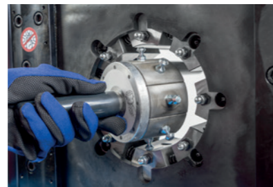
Die sets can be installed into the master dies with a QuickChange-tool one set at a time.
